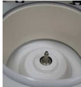
Motor shaft and chamber Figure. 10-1 (FC5515)
