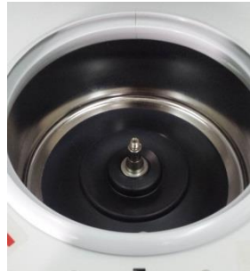
Motor shaft and chamber Figure.10 (FC5515R)
